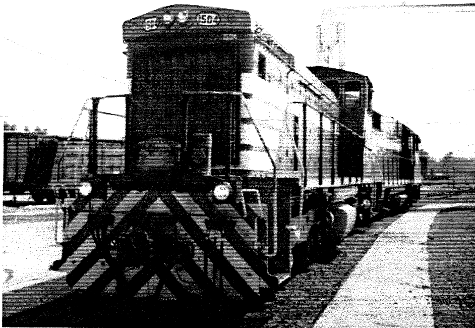
ABOVE: Fordyce & Princeton SW1500 #1504 and Arkansas, Louisiana & Mississippi GP28 #1812 are sitting at the shops in Crossett, Arkansas. The SW1500 just received ditch lights. Photo by Danny Schueth.
