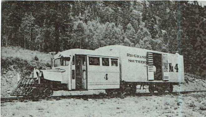
GEESE NOS. 3, 4 & 5 looked like this after being rebuilt in 1946 with schoolbus-type passenger body. No. 4 is shown near Vance Jct., Colorado in 1946. Photo: John W. Maxwell.
