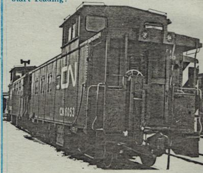
Narrow guage caboose of the Newfoundland Railway at the railway's main terminal, in St. John's, Newfoundland. Note the location of handrails and ditch lights. Perhaps someone could superdetail a caboose based upon this picture.
